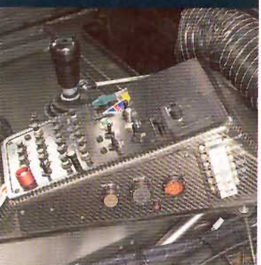
Shifty business: gears selected via a H-pattern shift for ALMS and Le Mans, sequential for FIA
